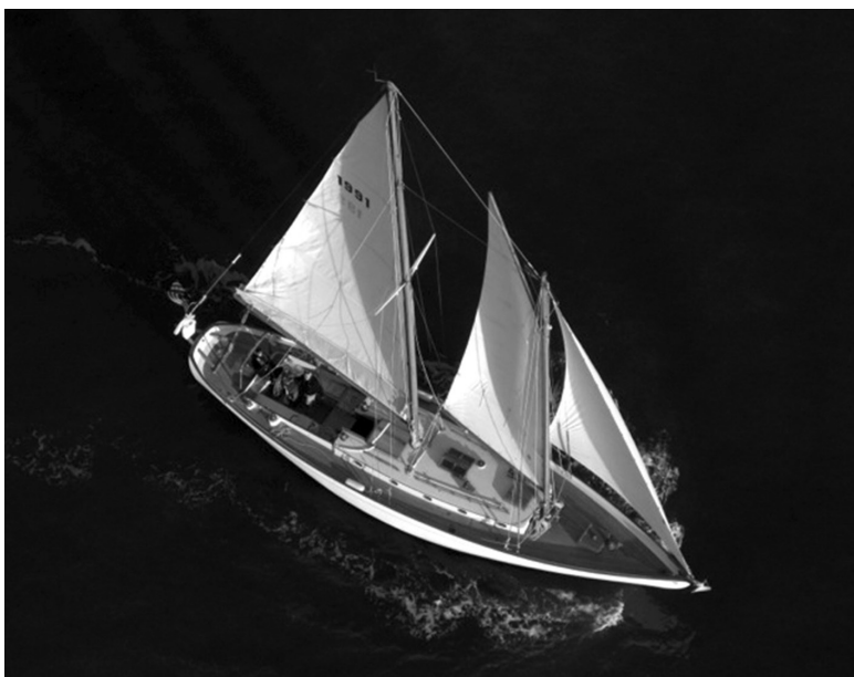
Gaff rig. This is a stunning aerial view of schooner Elizabeth Muir sailing with the gaff rigged foresail, the rig preferred by her present owners. The "gaff"—the wooden spar at the top of the (center) sail—is used to hoist it up. It provides more sail area and therefore more speed on certain points of sail than the staysail (triangular shaped sail not pictured here). The spacious cockpit is also shown. (Photo courtesy of Peter Haywood)
